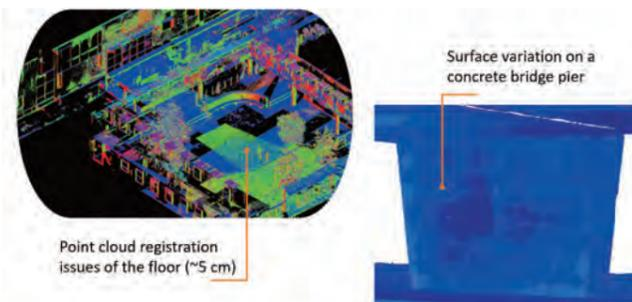
Figure 1. The point cloud on the left shows local irregularities in geometry pointing out data preparation errors such as misalignment. The one on the right shows surface variation of a bridge pier that can be monitored over time to spot abnormal behaviour.
