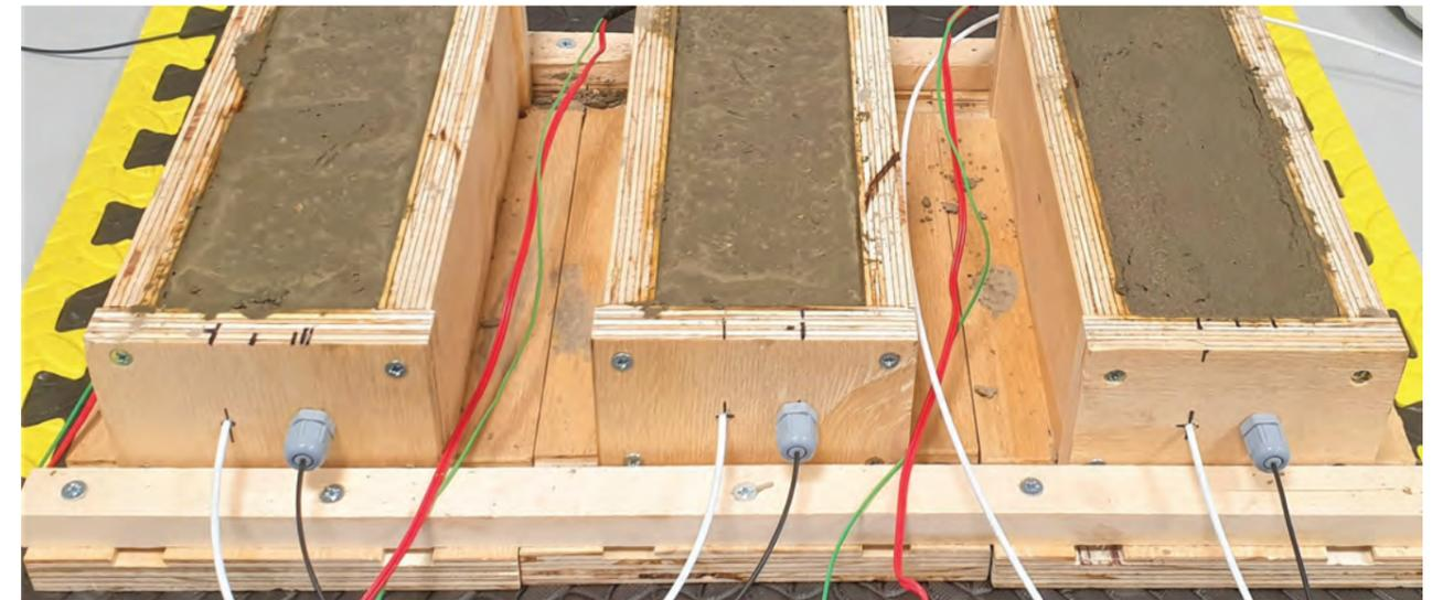
Concrete samples with embedded fibre optic sensors to measure strain and temperature
