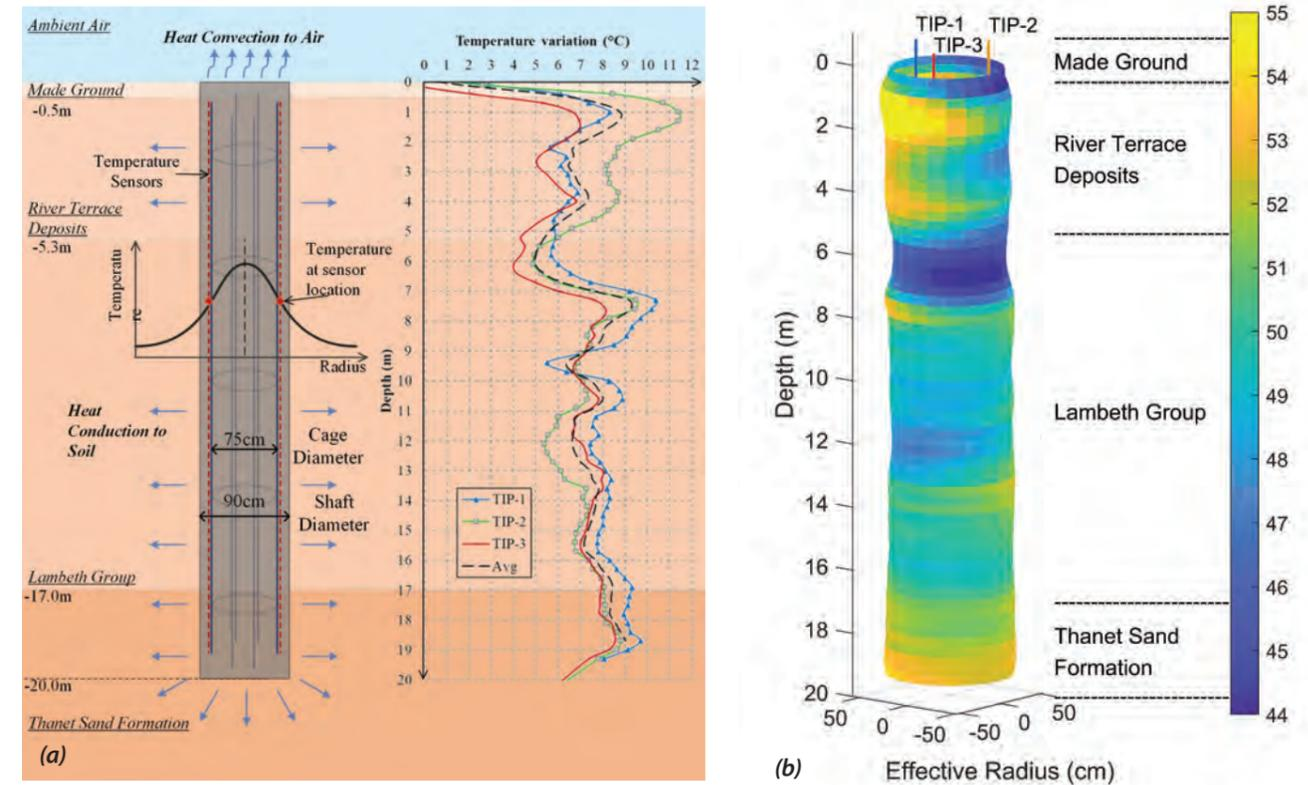
Figure 2. (a) Designed pile and recorded temperature profiles, (b) Generated 3D pile shape.
