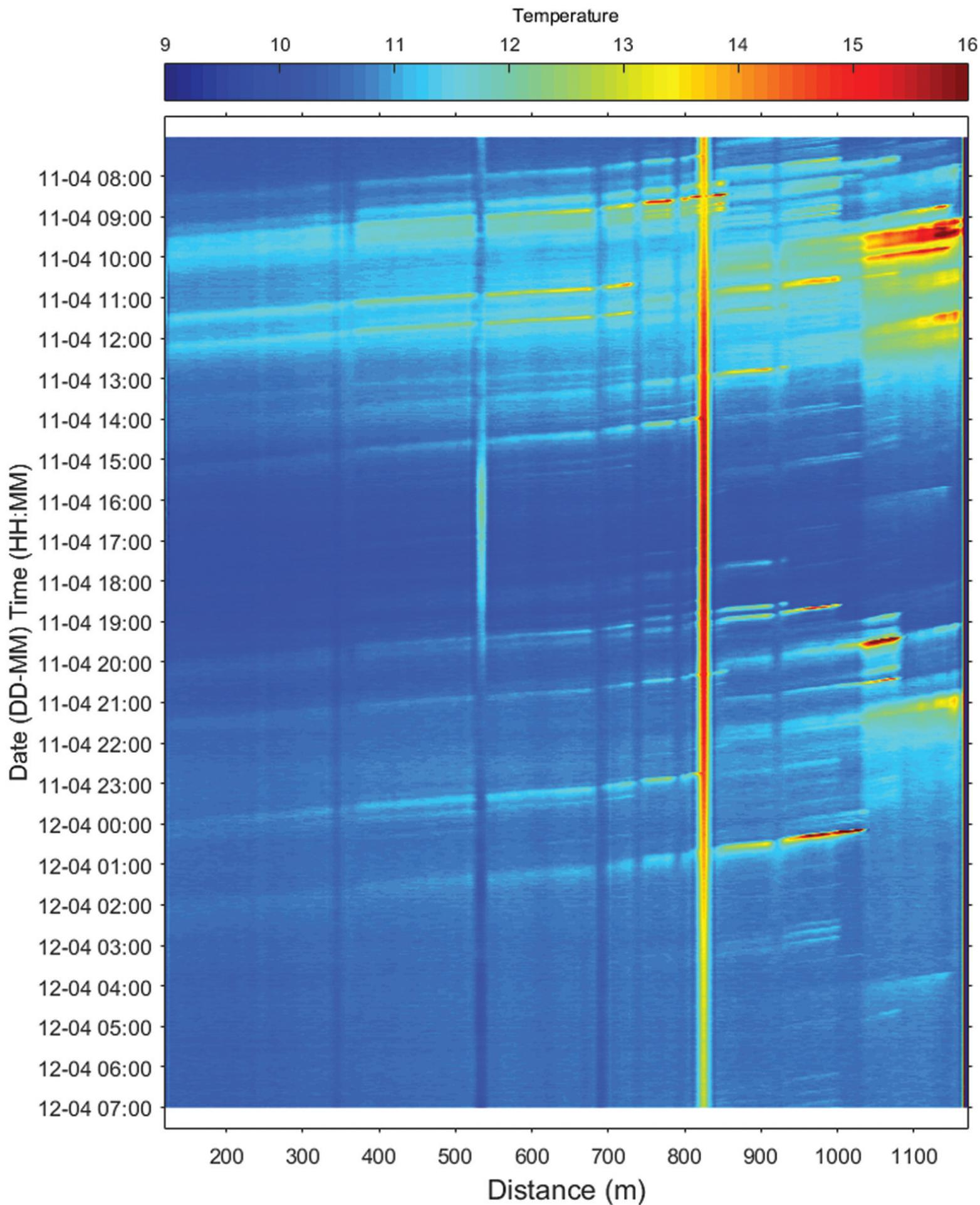
The graphic shows the temperature behaviour of the 1.2km of sewer being monitored over a 24-hour period. The deep blue colour is indicative of the ambient temperature of the sewer (10°C) in April. The green – yellow-red colours are of increasing temperature liquid joining the sewer from domestic connections, with flow in the sewer moving right to left. The (mostly) red vertical line is the air temperature inside a manhole, reaching around 16°C. Courtesy of Dr Y Rui
