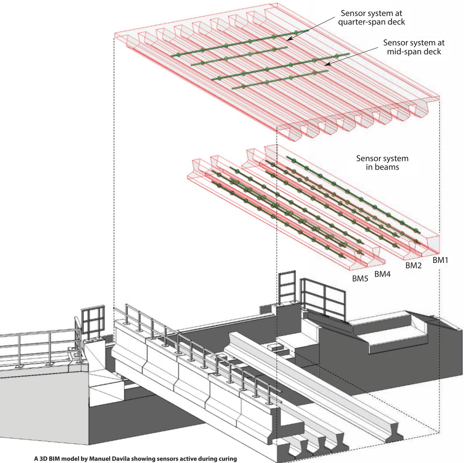
A 3D BIM model by Manuel Davila showing sensors active during curing in concrete rail bridge instrumented by CSIC in Staffordshire. For the full case study see page 19
